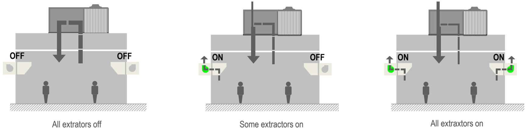
When the extractor hoods are activated the unit manage the fresh air damper to compensate the extraction air
